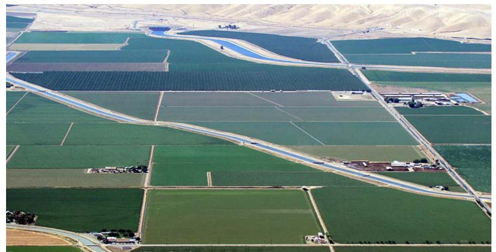
From top to bottom, 1-5. The California Aqueduct which ships water from the Delta to Southern California. Next is the Central Valley Project. At the bottom is a local canal.
