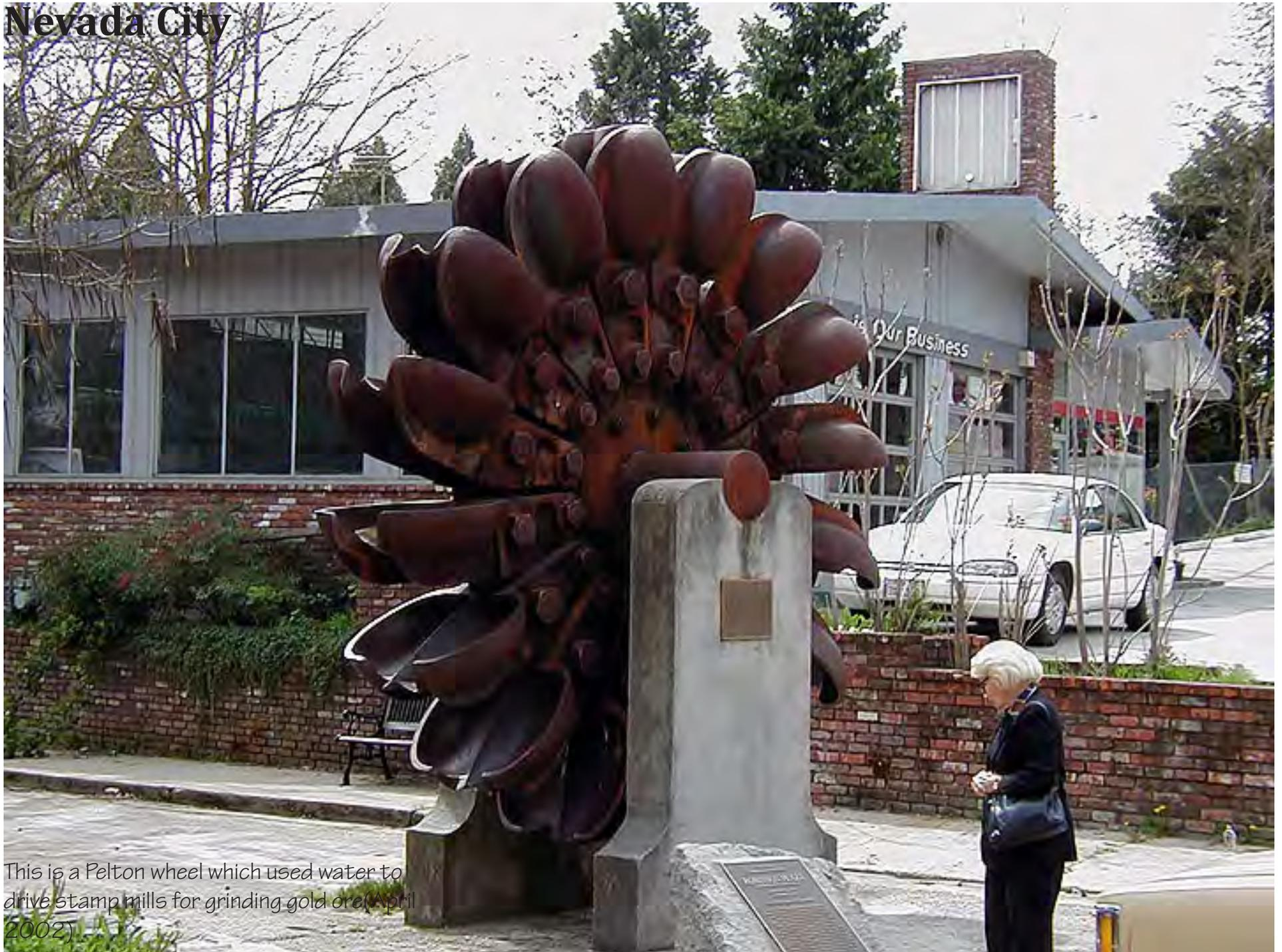
This is a Pelton wheel which used water to drive stamp mills for grinding gold ore (April 2002)
